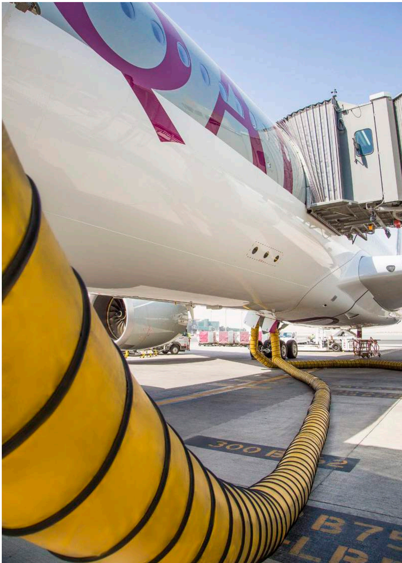
Providing pre-conditioned air to Qatar Airways aircraft
